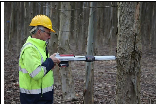
Figure 119: Collecting a Resi-trace at breast height (1.3 m above the ground). (Sylva Systems®.)
