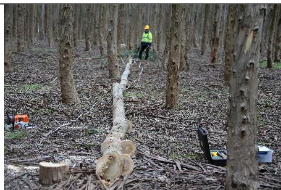
Figure 100: The sample discs sitting proud of the stem at the sampling point. (Sylva Systems®.)
