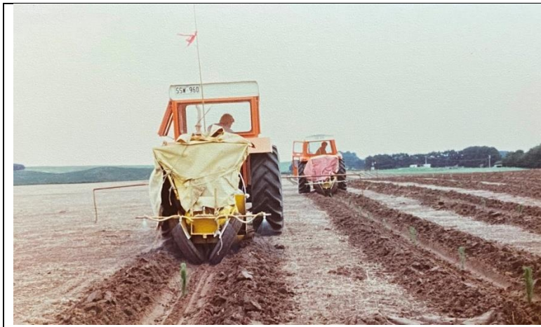
Figure 26: Pine planting machines in 1979 planting an ex-pasture site. Note the application of herbicide in the same pass (photo by DJ Geddes®).
