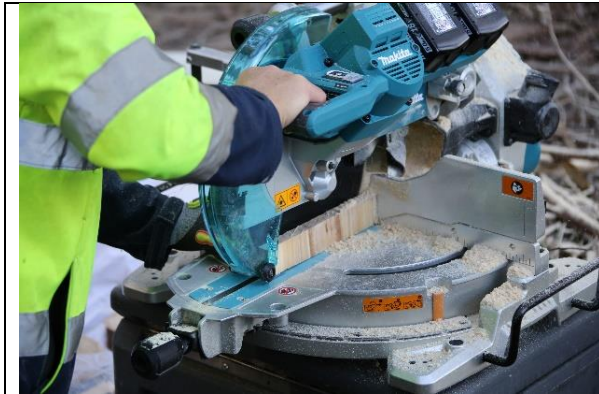
Figure 101: A compound mitre radial arm saw used to cut discs in half and to recover NIR analysis sample strips. (Sylva Systems®.)
