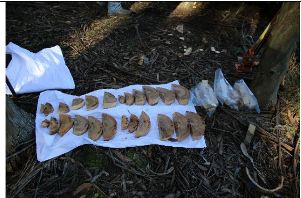
Figure 102: A set of sample half-discs from four trees and bagged NIR samples (one tree per bag). (Sylva Systems®.)
