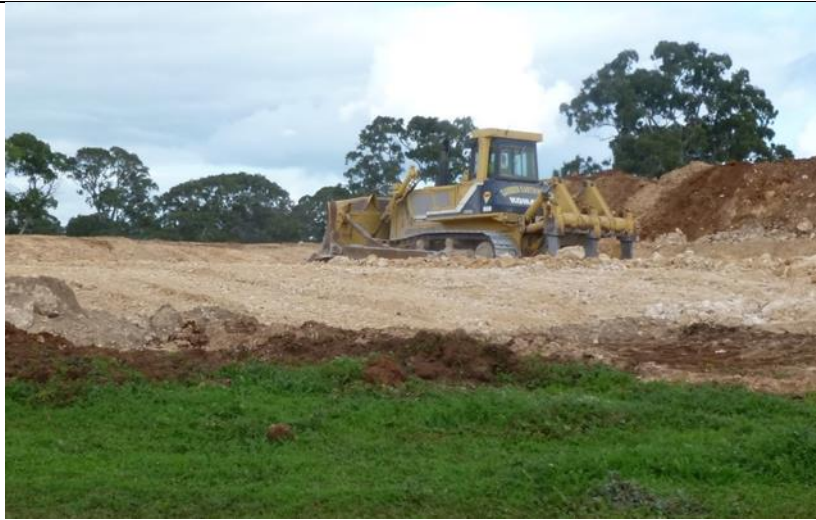
Figure 17: Raising road making materials (gravel) in a farm quarry (Photo by DJ Geddes®)
