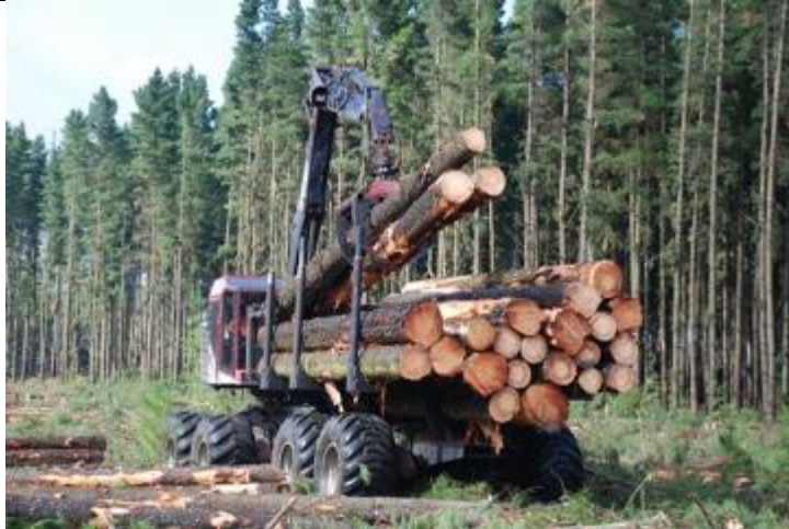
Figure 9: A forwarder loading large diameter logs from an older age softwood clear fall (Photo by LJ Parsons®)
