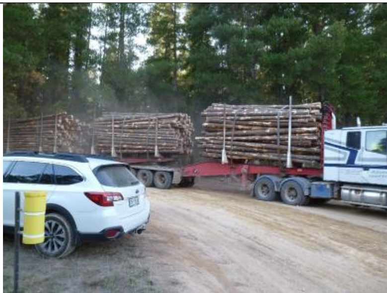
Figure 12: A B-double log truck with small diameter logs from a softwood T2 (Photo by DJ Geddes®)
