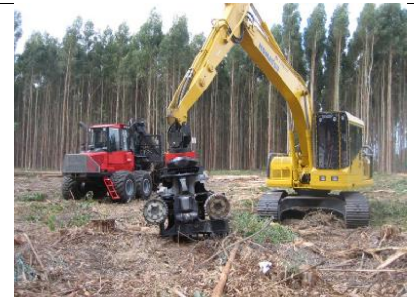
Figure 8: Forwarder and harvester at a hardwood clear fell (Photo by DJ Geddes®)
