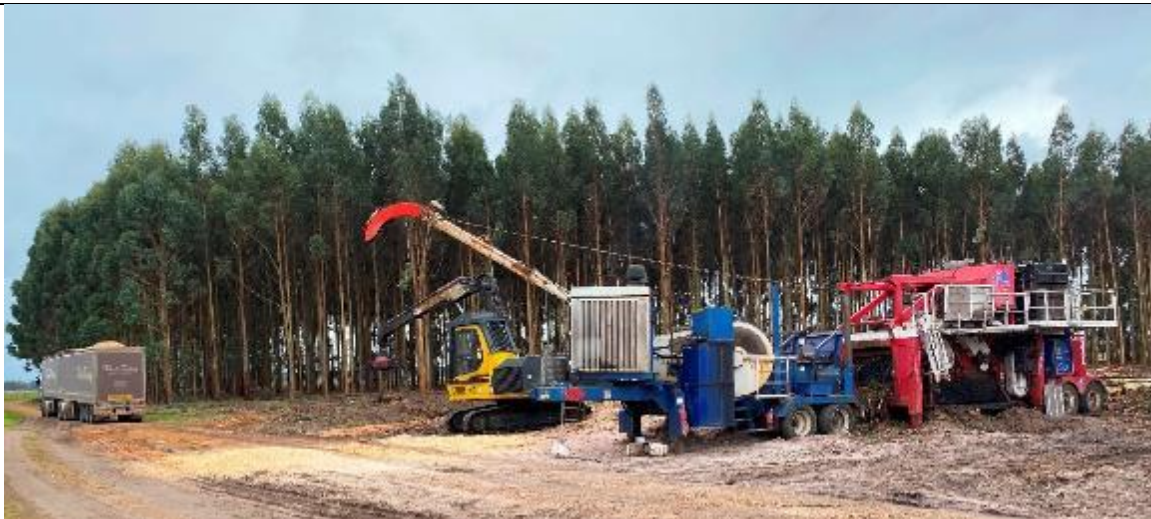
Figure 2: A WTC operation in a farmer owned hardwood plantation, showing a mobile chipper, a loader and a chip truck (Photo by DJ Geddes®)
